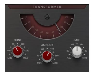
The distortion meter is an indication of the THD (Total Harmonic Distortion) of the signal.
